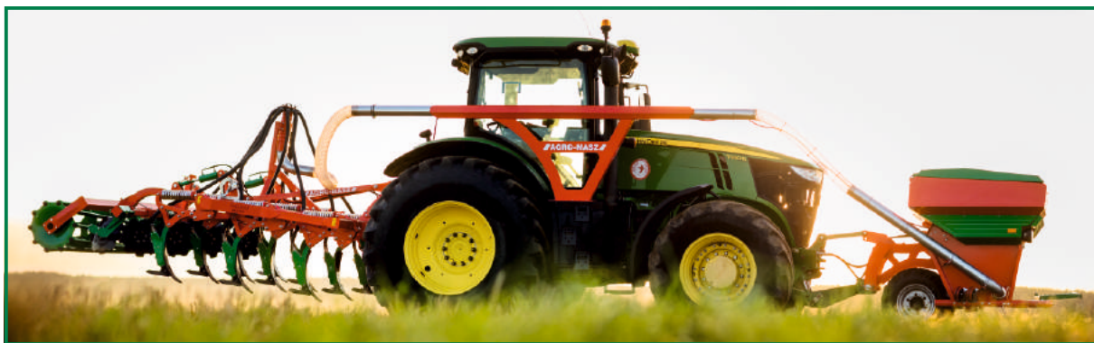
IKAR + RUNNER - set for simultaneous cultivation and soil fertilisation
